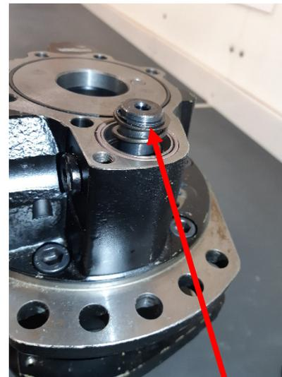
Valve with spring - correct position
